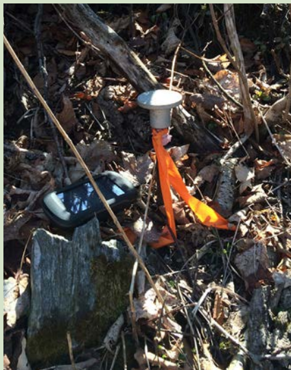
A well-marked boundary line includes painted blazes on trees, a rebar pin at each corner, and signage indicating the owner.
