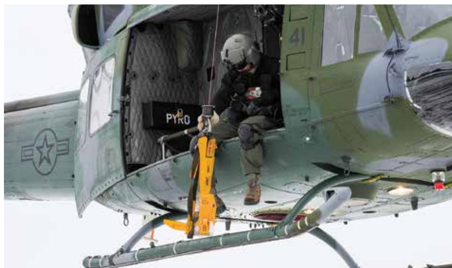
Preparing to lower a "jungle penetrator," a mechanical system used to resupply Pat and Stony.
